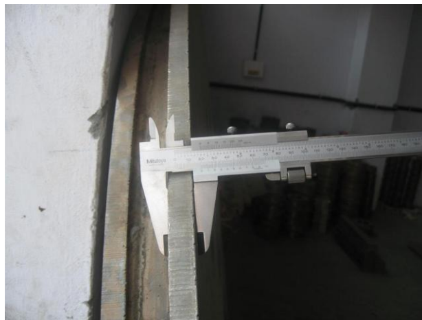
The thickness of the plate for making Steam jackets is 20mm Thick.
