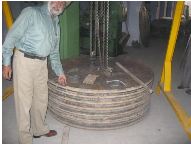
Steam Jackets to be fitted in the Cooker Drum
