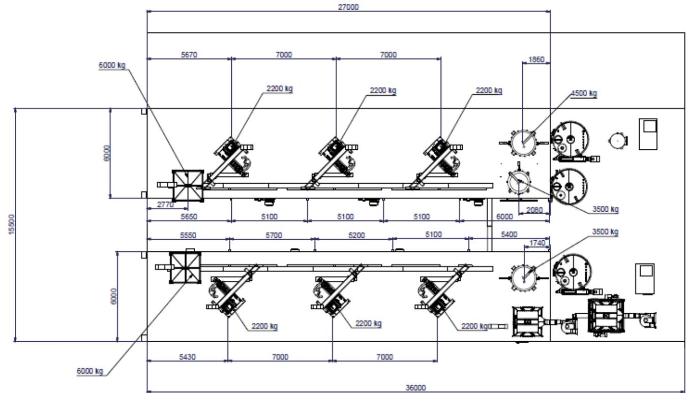
**Enclosure no. 4b: Dispositional Layout, Illustrative Scheme EP2-5(FS1010+FE1000+FS1010), incl. filtration**
